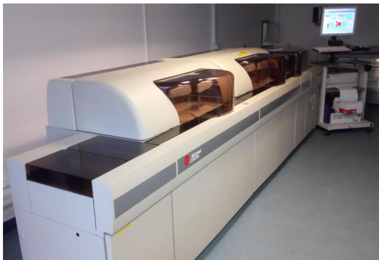
Figure 1: Beckman Coulter AU5400 Series Clinical Chemistry Analyser
