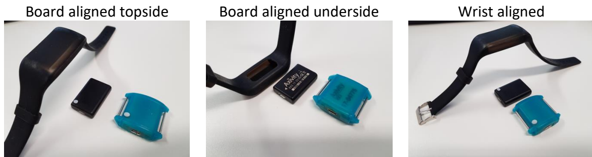
Figure 1 | Picture of first and second generations of Axivity AX3 enclosures used in UK Biobank (2013-2015). The turquoise blue outer case (here, without strap) shows the first-generation enclosure of the inner puck (yellow, faintly visible inside), while the black puck with silicone band shows the second-generation enclosure.
