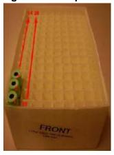
**5.3:** The saliva sample tube has a larger inner rack within the transport rack to ensure that the larger tubes are transported safely
