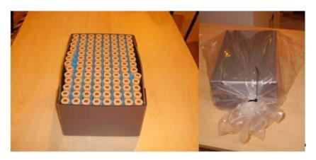
**5.5:** On the two short sides of the transport box are placed a cool pack and a spacer (see figure 4). The cool packs are kept in the freezer for at least 24 hours before use and are taken out 30 minutes before being used each day.
