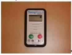
**7.2:** The co-ordinating centre configures the dataloggers to automatically begin recording, this is done before they are sent out to the assessment centre. Therefore the assessment centre does not need to press the start button. A symbol of a sun will be present on the datalogger screen to indicate it is set to automatically begin recording (figure 9).
