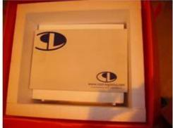
**5.7**: A third spacer is placed on top once the sample racks are all loaded and the third cool pack is placed on top of the spacer (figure 6).
